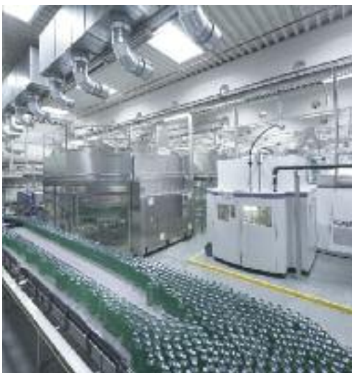
Römerquelle is the first company in the world to use an InnoPET Blofill stretch blow moulding machine/filler monoblock with integrated preform sterilisation for the production and filling of its PET bottles.
